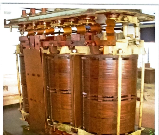
16 MVA, 33 KV / 400 V Furnace Transformer active part
