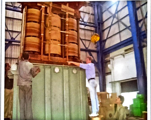
12.5 MVA 33/11 KV Power Transformer manufactured coils active part tanking process
