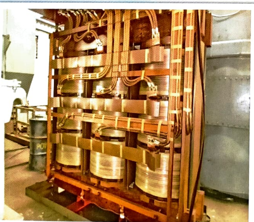
20 MVA 110/11 KV power Transformer active part
