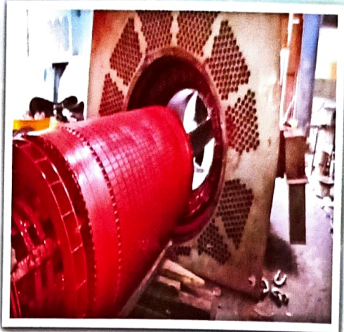
Assembling work of 3000 KW HT motor after rewinding of Stator & Rotor
