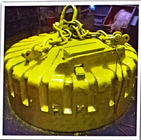
26 KW hot metal lifting circular magnet after rewinding
