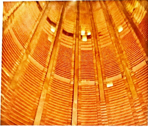
25 MVA, 110/11 KV Class Power Transformer Manufactured Coils
