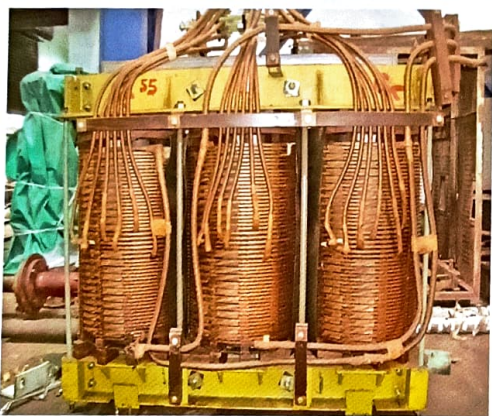
11 MVA Furnace Transformer active part
