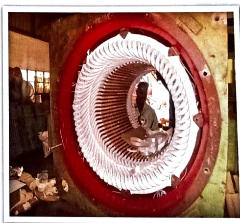
Rewinded motor stator of 2200 KW HT Motor
