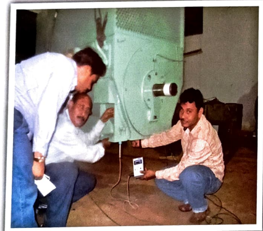
HT Motor vibration analyzing as per IS 12075
